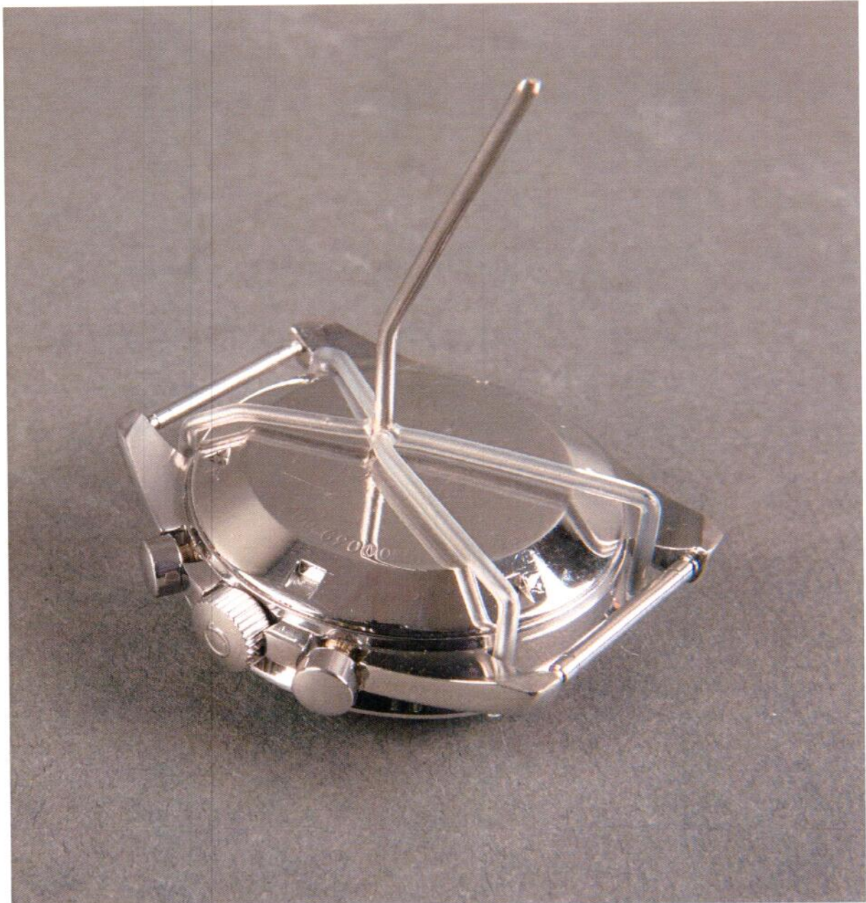
Figure 6: Back of the chronograph showing how the spider mount secures on the back.
